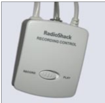
Figure 1: Smart Phone Recorder Control by Radio Shack feeds the signal from the phone line to the sound card in a Linux computer.
