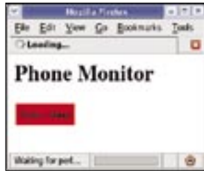
Figure 4: The listener verifies that the line is busy and displays a message.
