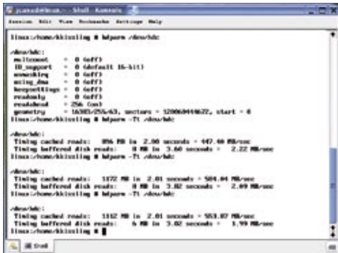
Figure 1: “hdparm /dev/hdc” without command-line options tells you which disk and drive features are currently enabled.
